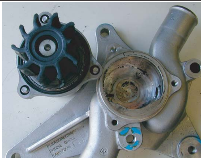
Figure 6-10 Failed Raw Water Pump Impeller
