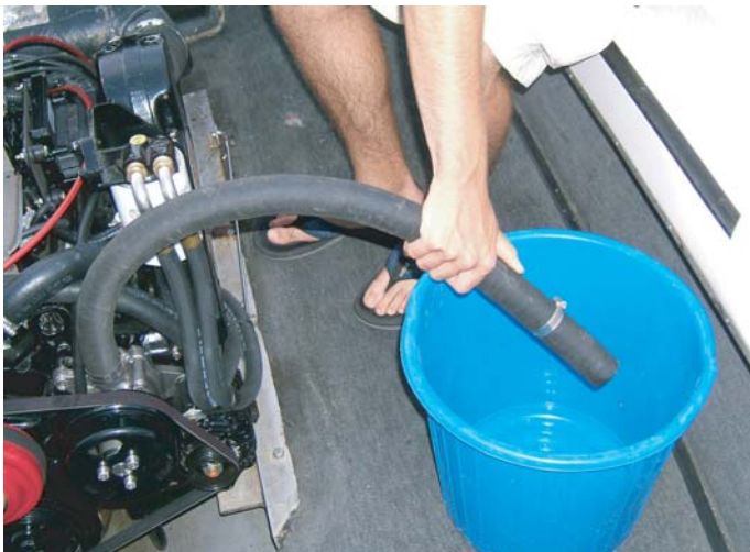
Figure 6-9 Raw Water Pump Volume Test
